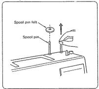
The spool pins are used for holding the spools of thread when feeding thread to the machine.
